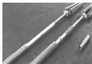
(c)在导电杆上设置绝缘件
